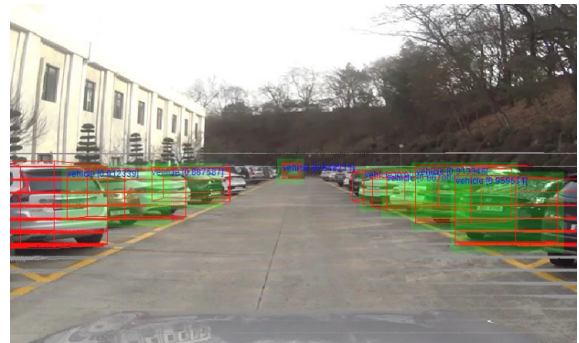
FIGURE 10. Result of multiple-object detection with 3D LIDAR and vision.
