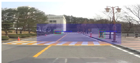
FIGURE 19. Result of pedestrian detection with 3D LIDAR and vision.
