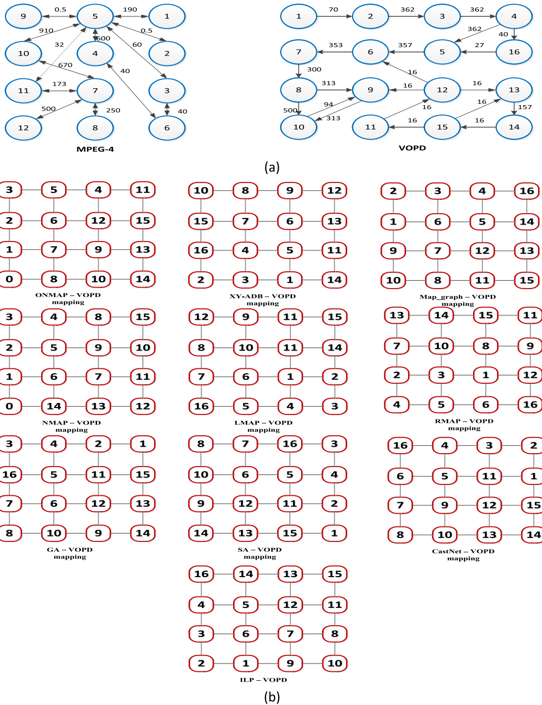
FIGURE 8. Mapping results of different application mapping algorithms (a) Task graph of MPEG-4 and VOPD (b) VOPD mappings.
