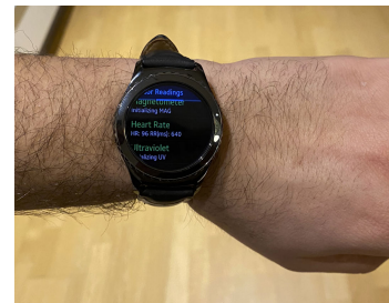
FIGURE 5. The image of working data collection application developed for Samsung Gear smartwatches on Tizen Wearable 2.2 API.
