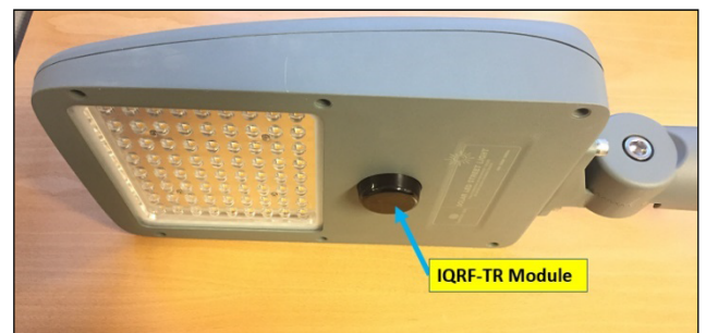
FIGURE 6. The attached IQRF-TR on the streetlight.
