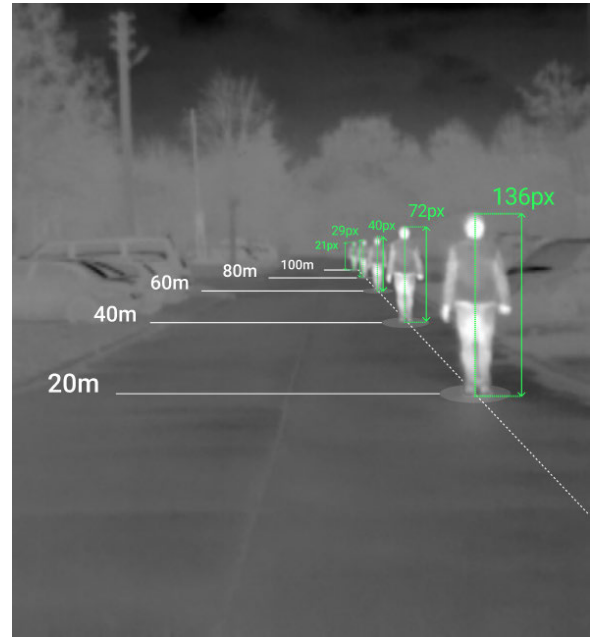
FIGURE 8. Pedestrian height distribution per distance.
