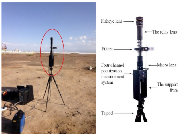
FIGURE 7. All-sky polarized skylight pattern imaging device.
