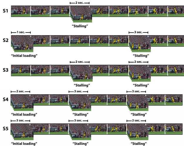
FIGURE 4. Freezing levels of distortion for scenarios S1 – S5.
