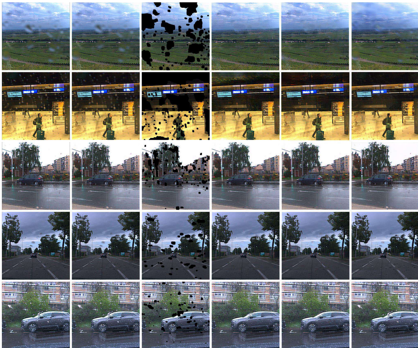
FIGURE 10. From left to right in each row: original sub-aperture image, enhanced image, masked image, recovered image with Edge Connect, recovered image with DFNet, recovered image with DeRaindrop [4].
