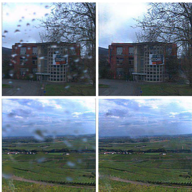
FIGURE 1. Left: The central images in the image arrays captured by the light field camera. Right: The recovered images which eliminate raindrops by binary masks, enhanced images, and image inpainting.
