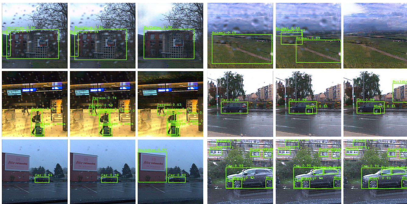
FIGURE 12. The object detection results of the original sub-aperture images, enhanced images, and recovered images, from left to right of each scenario.
