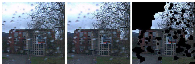
FIGURE 7. Left: the original sub-aperture image. Center: the refocused image processed by a high-pass filter. Right: the masked image.
