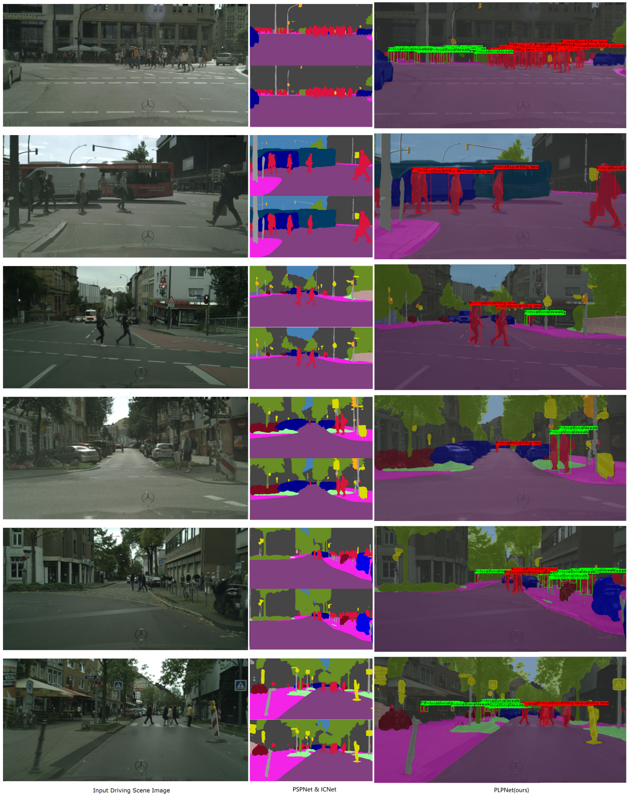
FIGURE 6. Comparison of P-LPN with semantic segmentation models (PSPNet (upper image) and ICNet (under image) in the middle column).
