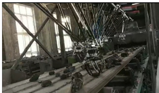
FIGURE 2. Manipulators pick up gangue in a mining factory by using X-rays.
