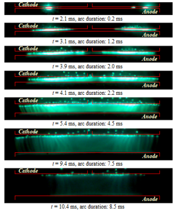
FIGURE 8. Arc behavior of parallel vacuum arcs. Split electrode worked as cathode with current of 18.9 kA.
