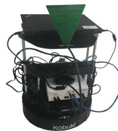
FIGURE 4. A TurtleBot robot equipped with USRP N210 and GNU Radio.
