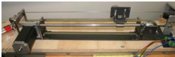
FIGURE 16. BassBot's pitch shifting mechanism. A system that uses a timing belt to drive a metal carriage to apply pressure across the string.
