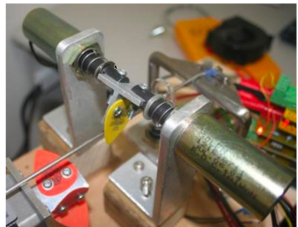
FIGURE 1. Push-pull picking mechanism. A simple configuration that uses two opposing solenoids to pluck the string.
