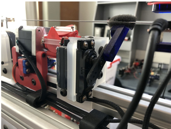
FIGURE 11. MechBass' damping mechanism. A servo pushes a piece of felt to mute the string.
