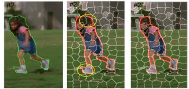
FIGURE 6. Optimize object contour by the boundaries of matched superpixels. The predicted object contour (green line in the first column) is optimized by two matched superpixels (yellow circles in the second column) to produce better segmented result (red line in the third column).
