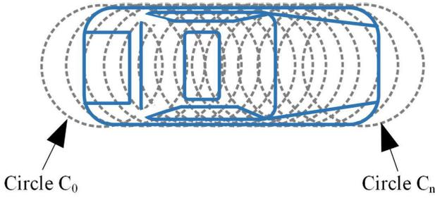
FIGURE 3. Vehicle representation by infinite dynamic circles.
