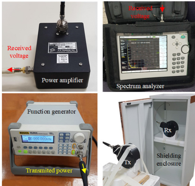
FIGURE 10. SE measurement setup using the proposed antenna.
