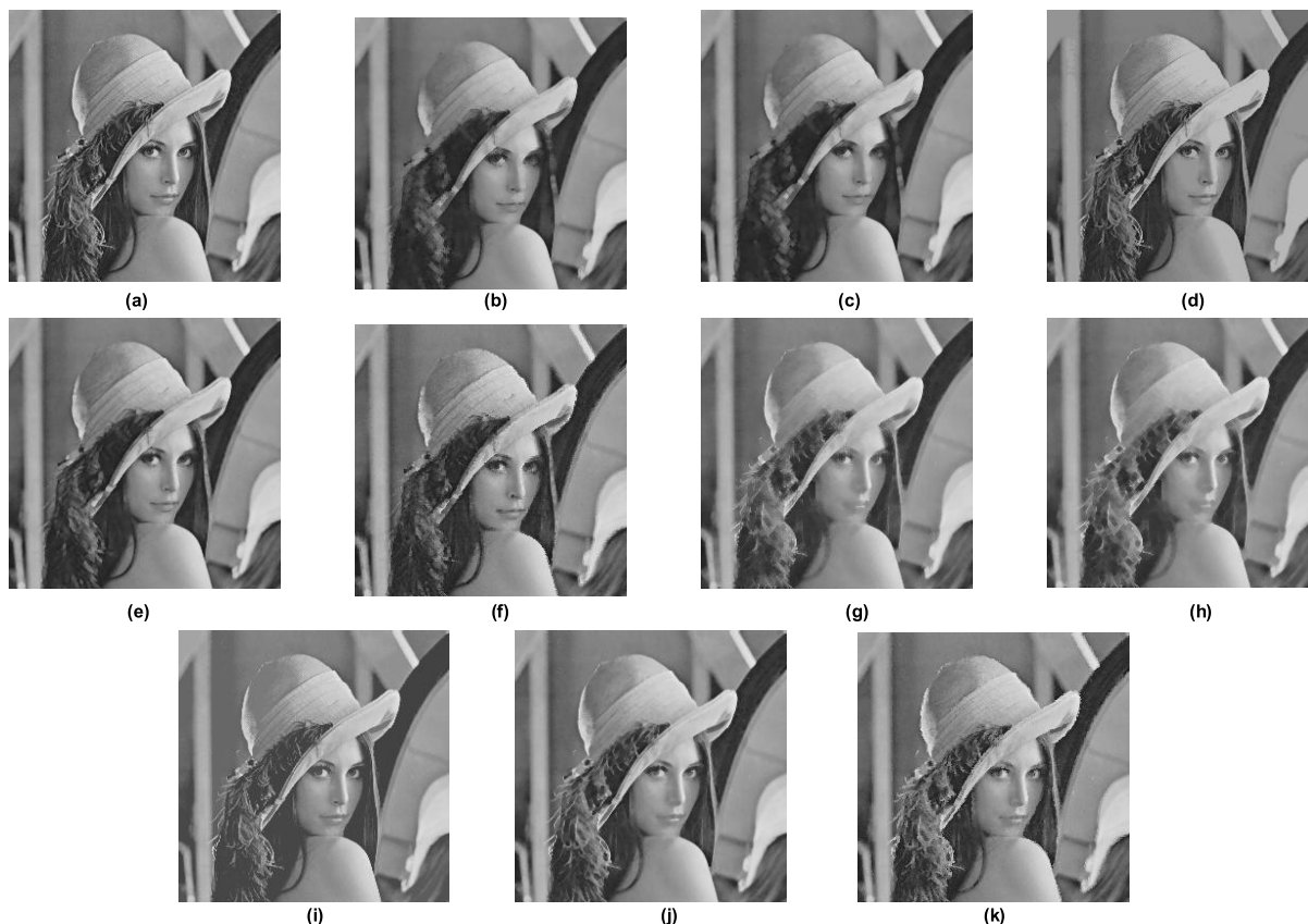
FIGURE 13. Results of opening and closing operations with different structuring elements on grayscale image. (a) Original image. (b) Result of opening operation with cross-shaped structuring element. (c) Result of opening operation with circular structuring element. (d) Result of opening operation with Pinoli's [16] adaptive structuring element. (e) Result of opening operation with Landström's [20] adaptive structuring element. (f) Result of opening operation with proposed adaptive structuring element. (g) Result of closing operation with cross-shaped structuring element. (h) Result of closing operation with circular structuring element. (i) Result of closing operation with Pinoli's [16] adaptive structuring element. (j) Result of closing operation with Landström's [20] adaptive structuring element. (k) Result of closing operation with proposed adaptive structuring element.
