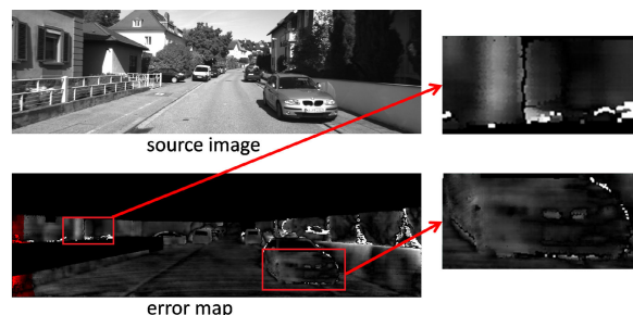
FIGURE 1. The disparity estimation results of the latest method in ill-posed areas. The error map scales linearly between 0 (black) and 5 (white) pixels error. As shown in the enlarged area of the image frame, there is a large error in disparity estimation in the reflected area of vehicle and wall.
