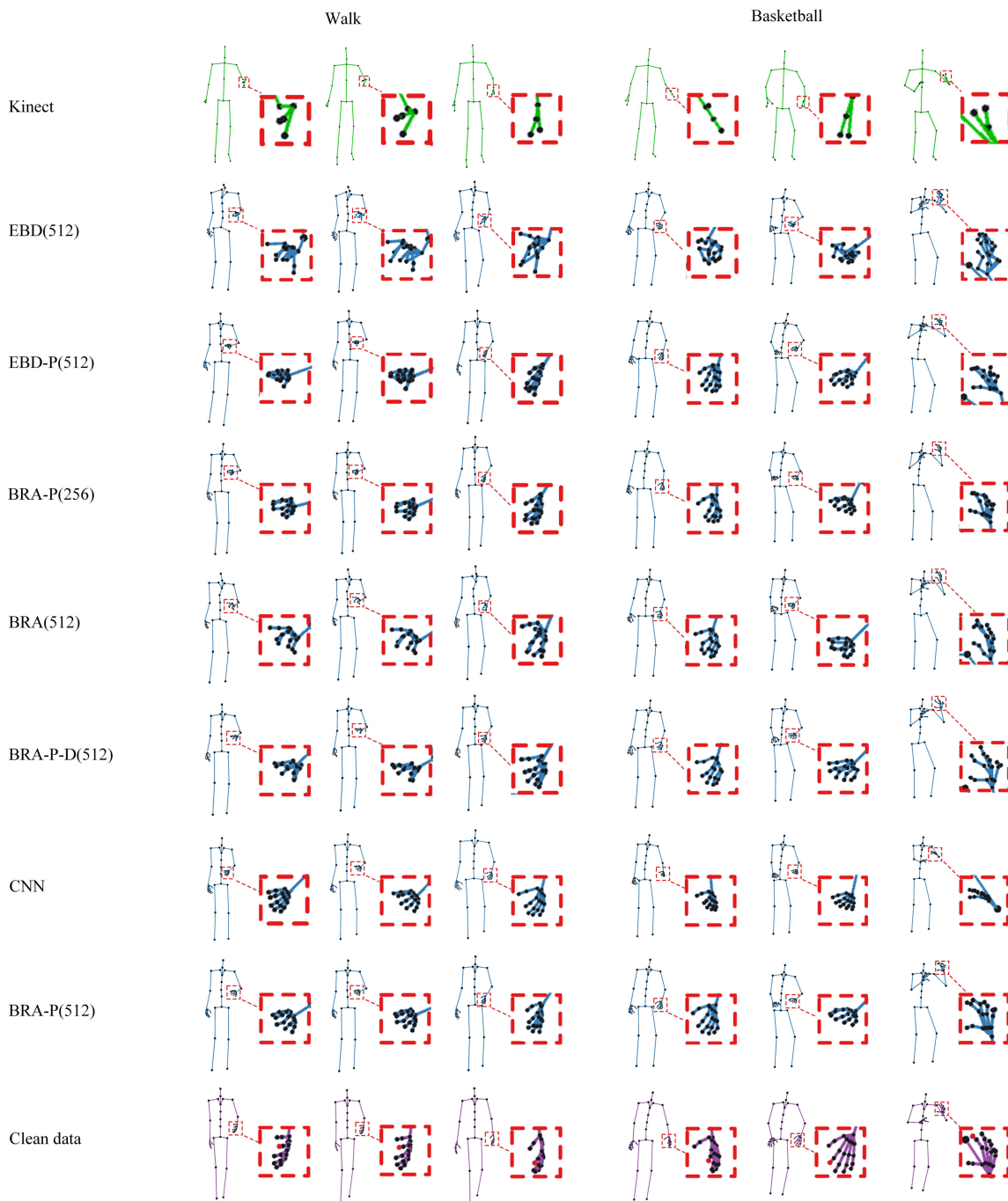
FIGURE 10. Key frame sequence of the refinement results obtained via various approaches. The hand of each refined pose is circled and magnified for a clear comparison. The hand skeleton in raw data captured by Kinect is indistinct but should be clear in the refined pose, and the joint numbers of the two spines are also different. The results show that the spine and hand components of the results of BRA-P are more natural than its variants. CNN can produce a good skeleton topology, but the result is jittery. Readers can refer to the supplementary video for additional information.
