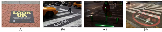
FIGURE 1. (a) Signage in Delaware, (b) Signage in NYC, (c) LED spotlight in Israel, (d) Ground flashlight in Seoul. Numerous pedestrian safety systems have been developed.
