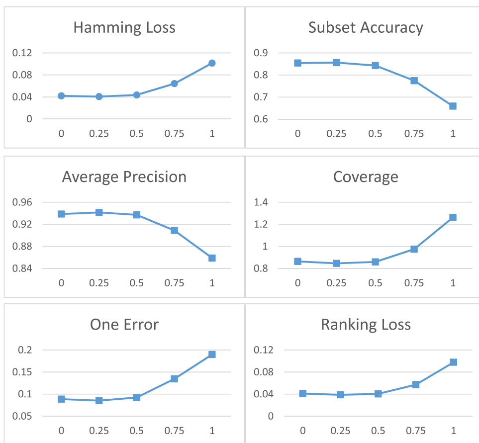
FIGURE 2. Six measurements of MF-EFP averaged over the 30 runs on the dataset I with different number of weights \alpha . The horizontal axis is the weights of the two scores based on features and neighbors, and the vertical axis represents the average measurement values by five-fold cross-validation.
