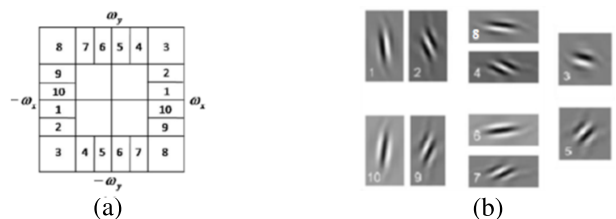
FIGURE 3. (a) Frequency-domain partition obtained from two level 2D ADTCWT decomposition; (b) Basis functions of 2-D ADT-CWT.
