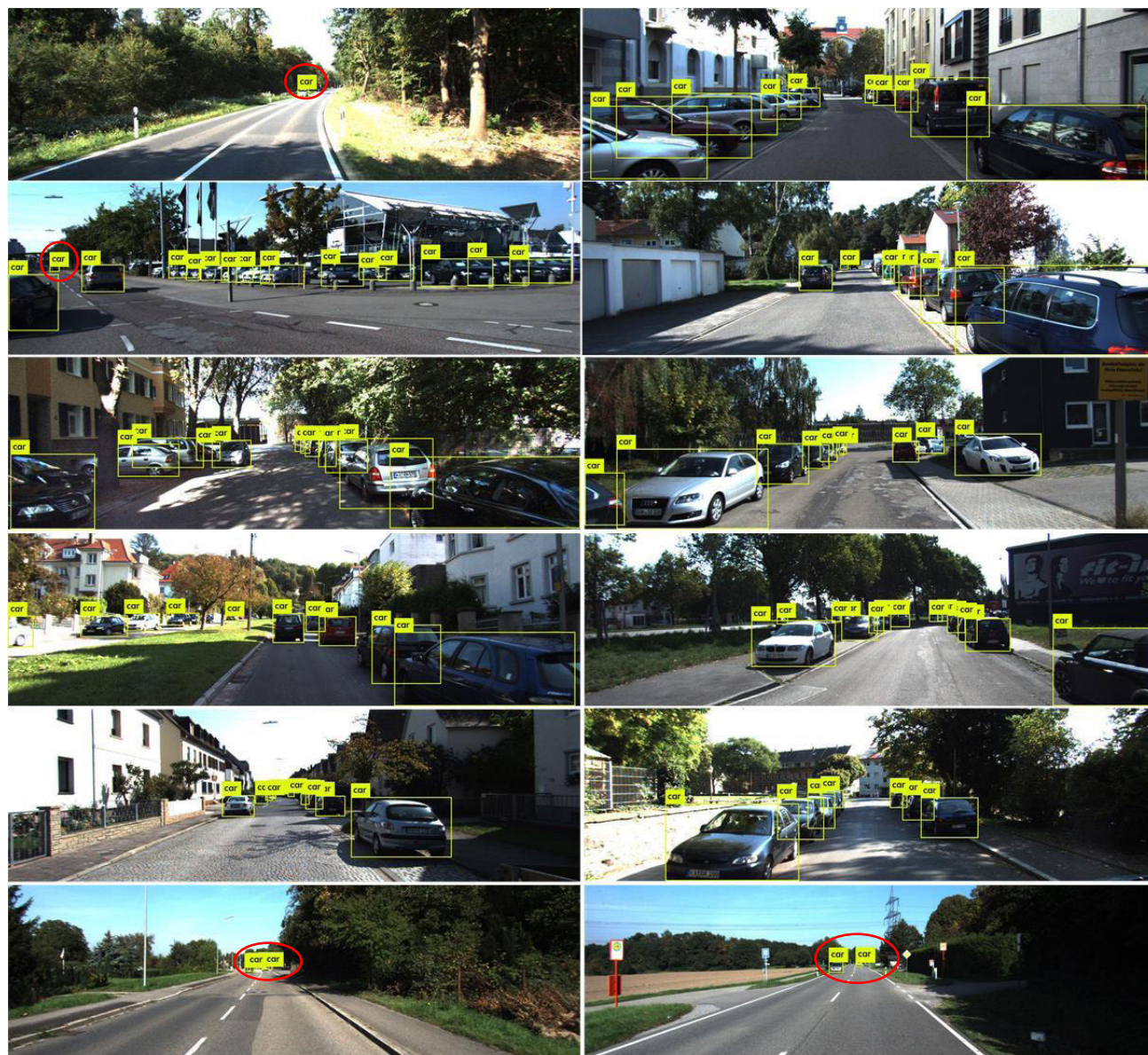
FIGURE 11. The test results of this algorithm are used on the KITTI test set. The red circles circle the vehicle detection results at a small scale. It can be seen that the algorithm in this paper can better adapt to the occlusion of the target and has a strong adaptability to the target's scale Capability, the detection of small targets is relatively stable, and it can better meet the actual needs of vehicle detection under complex traffic video.
