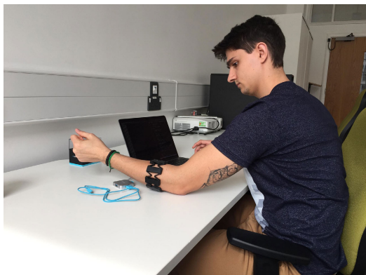
FIGURE 3. Data collection from a male subject via the Myo armband on their left arm.
