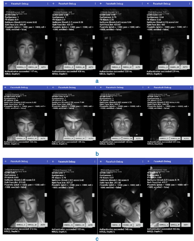
FIGURE 12. a. Snapshots from yaw angle position tests. b. Snapshots from pitch angle position tests. c. Snapshots from roll angle position tests.
