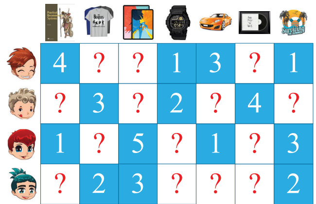
FIGURE 6. The matrix of different users and items. Each row represent a user, and each row represent every item in the catalogue.
