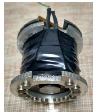
FIGURE 6. Polarized magnetic system physical prototype.
