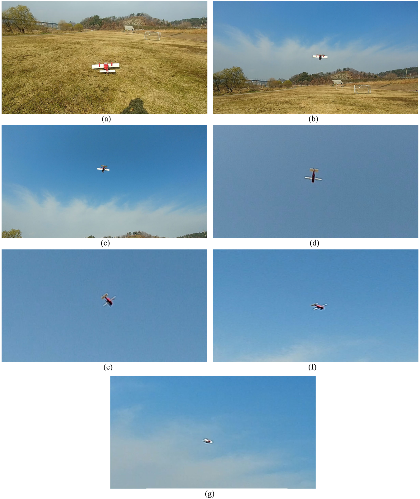
FIGURE 16. Outdoor flight experiment with wind disturbance: (a) prototype of the UAV; (b) vertical take-off; (c) hovering; (d) vertical flight; (e) forward transition; (f) horizontal flight after forward transition; (g) backward transition.
