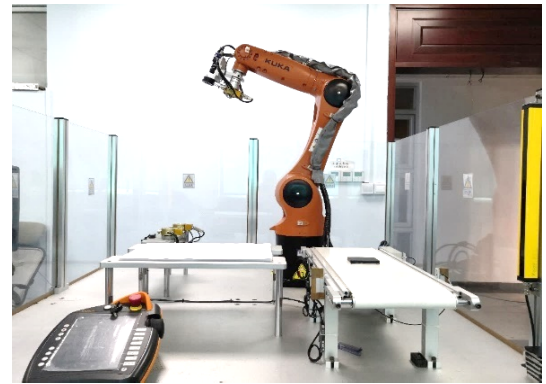
FIGURE 4. KUKA KR6R 900 SIXX industrial robot.
