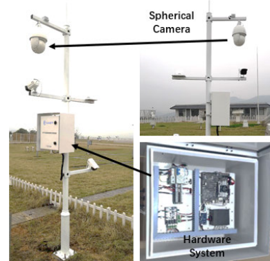
FIGURE 7. Our Observation and Classification System. This paper mainly uses the spherical camera and Jetson TX2 embedded platform.
