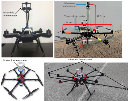
FIGURE 4. Top Left: Tri-Sonica ultrasonic anemometer attached to quadrotor [14]. Top Right: FT702 ultrasonic anemometer attached to hexarotor [15]. Bottom Left: DS-2 ultrasonic anemometer attached to hexarotor [12]. Bottom Right: FT205 ultrasonic anemometer attached to octorotor [49].
