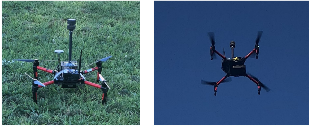
FIGURE 7. FT-205 wind sensor mounted on the DJI Matrice 100 sUAV to collect wind data during flight test.
