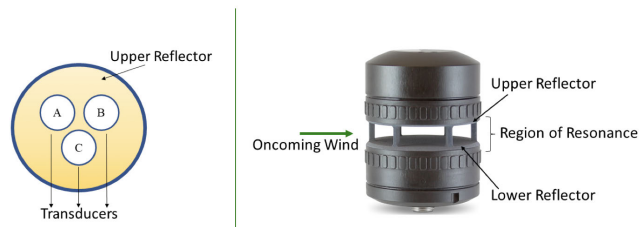
FIGURE 6. Left Image: Alignment of transducers on the upper reflector for an acoustic resonance ultrasonic anemometer. Right Image: Side view of the FT205 acoustic resonance ultrasonic anemometer.
