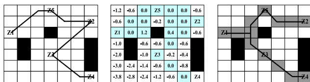
FIGURE 6. 2D Example of SMT and Improvement Table (a) Initial minimal spanning tree, (b) Improvement Table, and (c) The SMT after adding one Steiner node.
