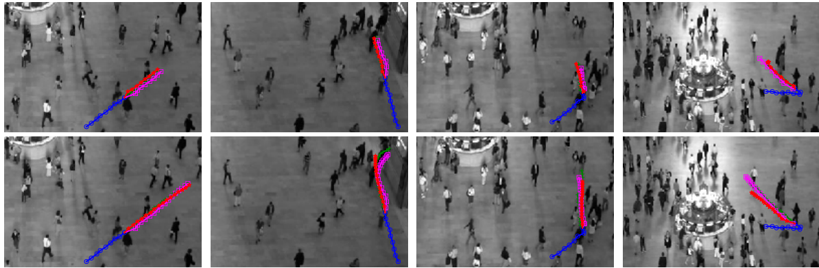
FIGURE 8. Prediction results of different prediction horizons: T_{ph} = 8 frames (first row) and T_{ph} = 16 frames (second row) on the Central Station test set. Colour codes: blue: input observed trajectories; green: ground truth trajectories; red: LVTA-8; pink: LVTA-16. The background scene in each subfigure is the first frame of the prediction phase.
