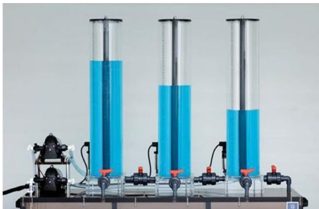
FIGURE 1. The three water tanks of TTS20.
