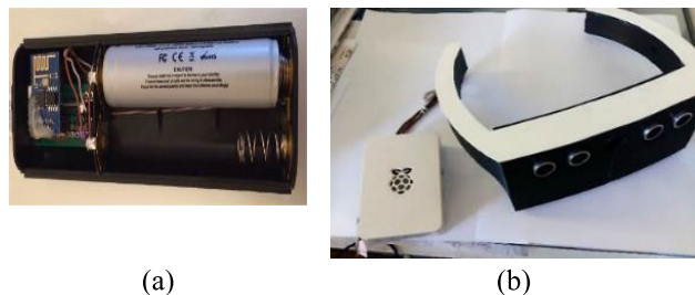
FIGURE 25. (a) fixed device and (b) pair of glasses used for indoor mapping and navigation.
