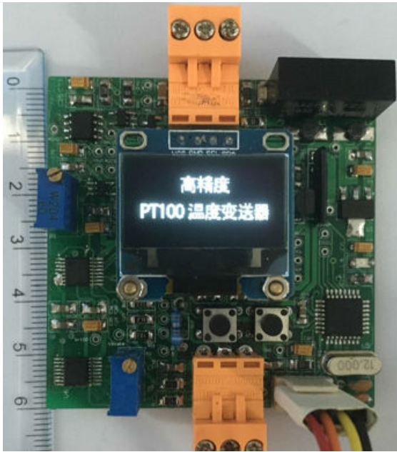
FIGURE 6. The designed temperature sensor using DCCS.
