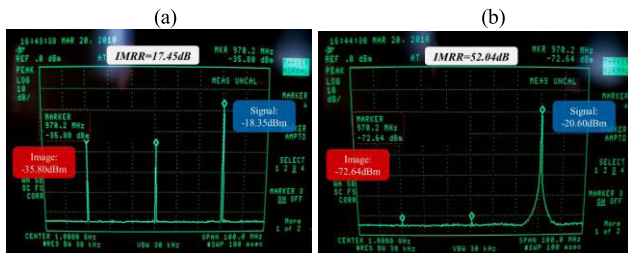
FIGURE 14. Single tone at 1030 MHz to verify the calibration performance for the ITRI TX module: (a) IMRR = 17.45 dB before preprocessing and (b) 52.04 dB after preprocessing.
