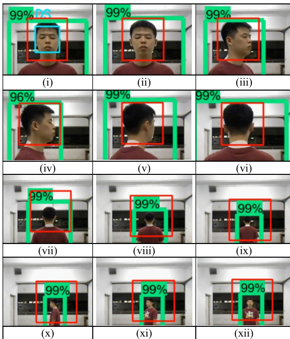
FIGURE 11. Performance evaluation of KCF with simultaneous FaceNet and SSD operations. (i) SH is respectively detected, recognized and tracked by SSD, FaceNet and KCF, (ii) FaceNet does not work, (iii)–(vi) different orientations of human are still successfully detected and tracked by SSD and KCF, (vii)–(ix) different distances of human are still successfully detected and tracked by SSD and KCF, (x)–(xii) different orientations at 8m between them are still successfully detected and tracked by SSD and KCF.
