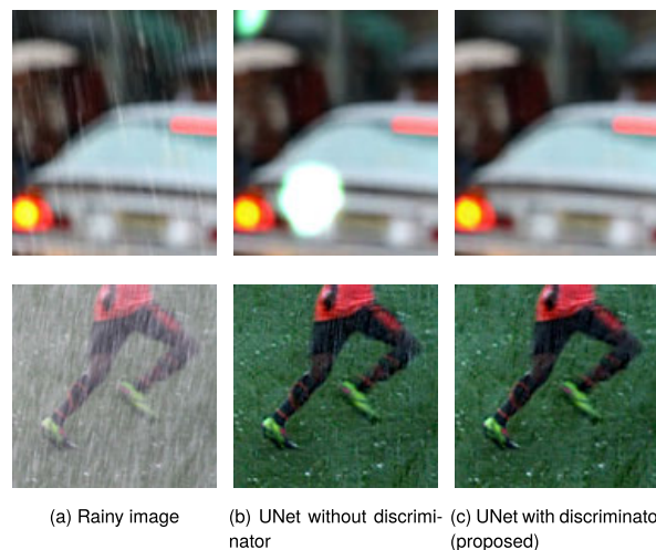
FIGURE 4. Comparison of two different networks. Top: Synthetic image. Bottom: Real-world image. (a) rainy image, (b) de-rained output of UNet without discriminator, (c) de-rained output of UNet with discriminator (proposed GAN-based network).
