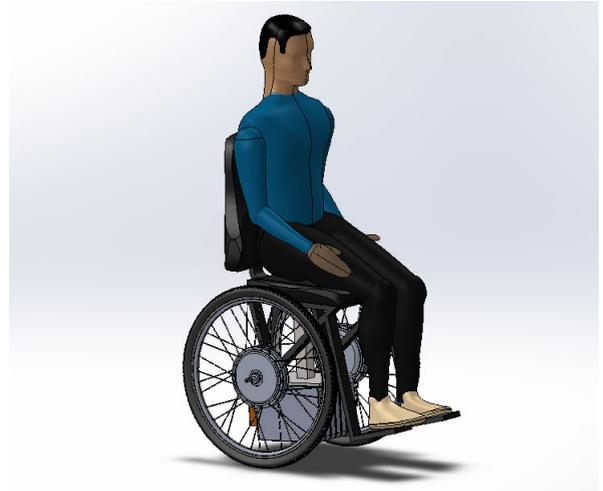
FIGURE 1. TWRW prototype.
