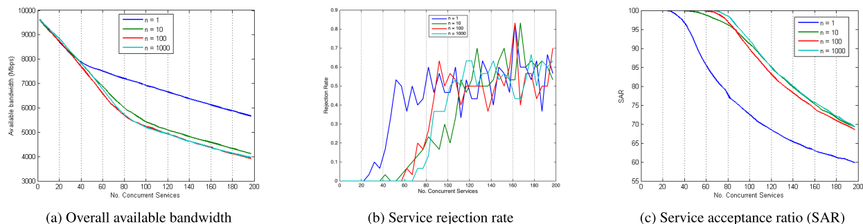
FIGURE 17. Impact of the number of alternative paths on network resources' utilization and SAR.
