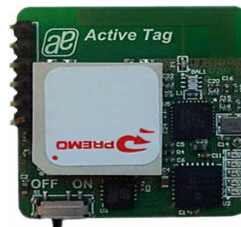
FIGURE 6. An active RFID Tag (containing an internal battery) [134].
