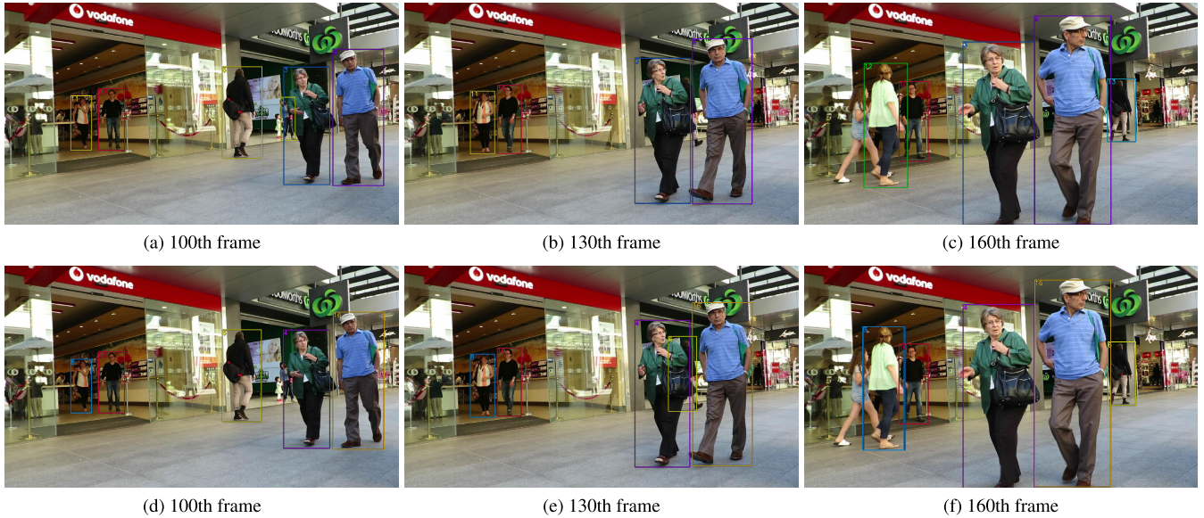
FIGURE 6. Tracking results on the MOT17-09-FRCNN dataset. In the top row, (a)–(c), present the results for JBNOT [20] and in the bottom row, (d)–(f) present our results for the same sequence. The man wearing a black jacket in the 100th frame is consistently tracked by our tracker. However, JBNOT fails to track the man because he is occluded by other objects.
