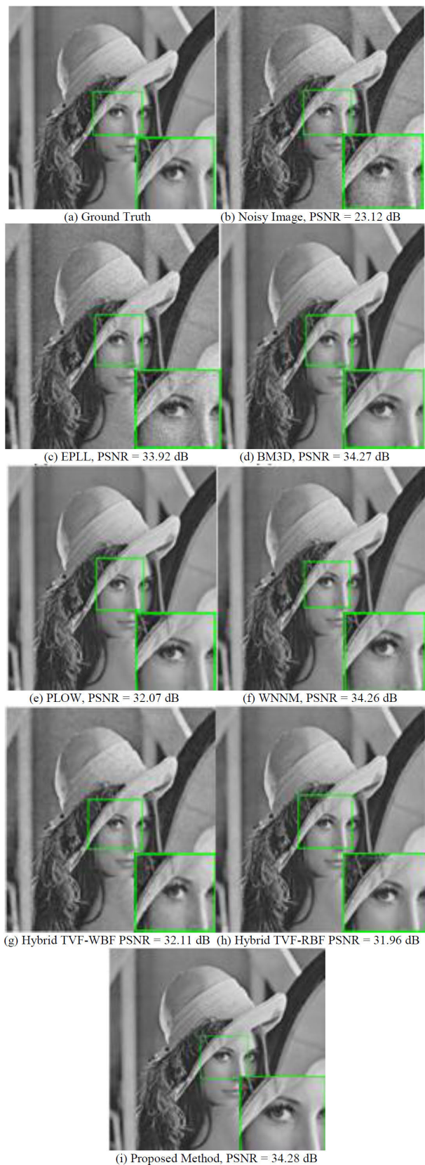
FIGURE 2. Subjective quality comparison of denoised images using different denoising methods on image Lena.
