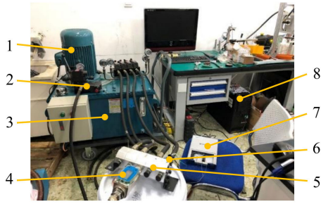
FIGURE 6. Experimental stand of the synchronous hydraulic motor. 1 Pressure gauge; 2 reversing valve and relief valve assembly; 3 fuel tank; 4 flow meter; 5 synchronous hydraulic motor; 6 acoustic sensor; 7 data acquisition card; 8 computer.
