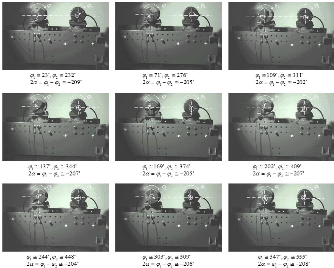
FIGURE 12. Phase difference with two co-rotating rotors in a vibrating system.
