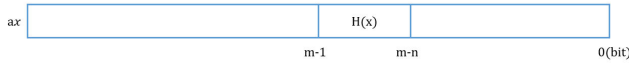
FIGURE 1. Multiply-shift hash, extracting bits m - n, \dots, m - 1 from the product ax as the hash value.
