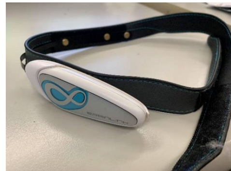
FIGURE 2. Head-mounted non-invasive EEG instrument-BrainLink Lite.
