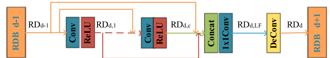
FIGURE 4. The structure of our RDB. Each RDB contains 16 \times 3 \times 3 convolutional layers, 1 \times 1 convolutional layer, and 1 \times 4 \times 4 deconvolutional layer.
