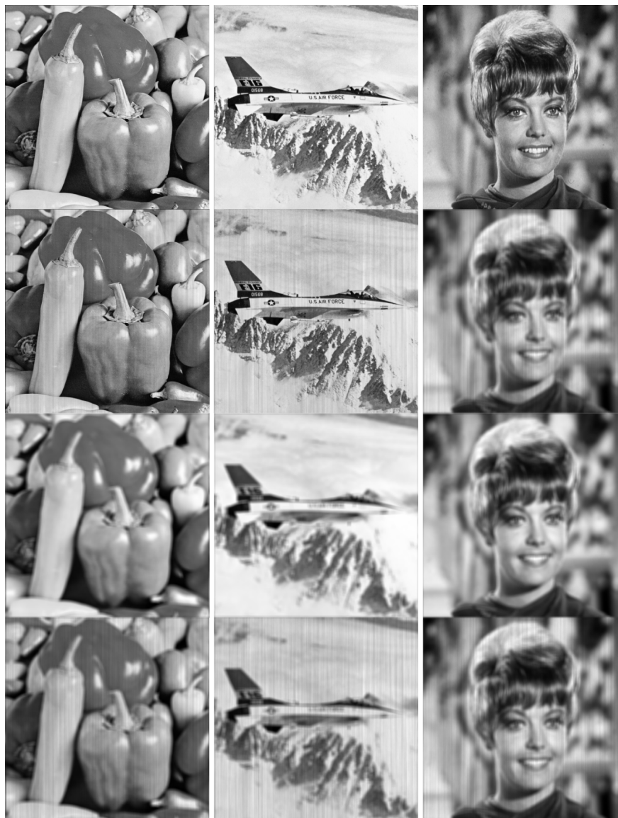
FIGURE 3. The top row: showing three clean images. The second row: showing images only affected by structured noise (stripes noise). The third row: showing images only affected by average blur (AB (10)). Bottom row: showing the images are affected by average blur and stripes noise.
